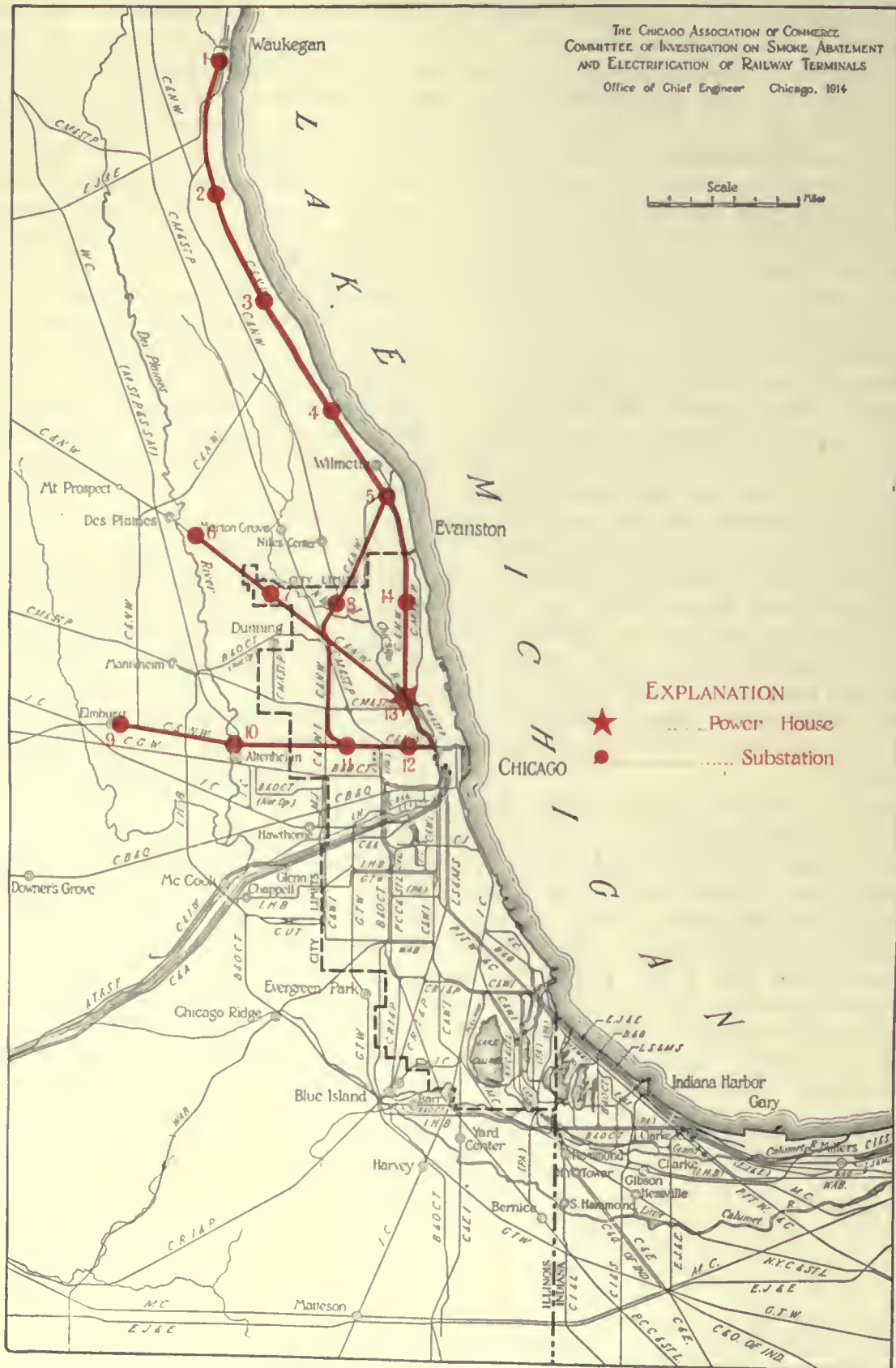
FIG. 684. LOCATIONS OF POWER STATION AND SUBSTATIONS FOR THE 600-VOLT D. C. SYSTEM. CHICAGO & NORTH WESTERN RAILWAY
